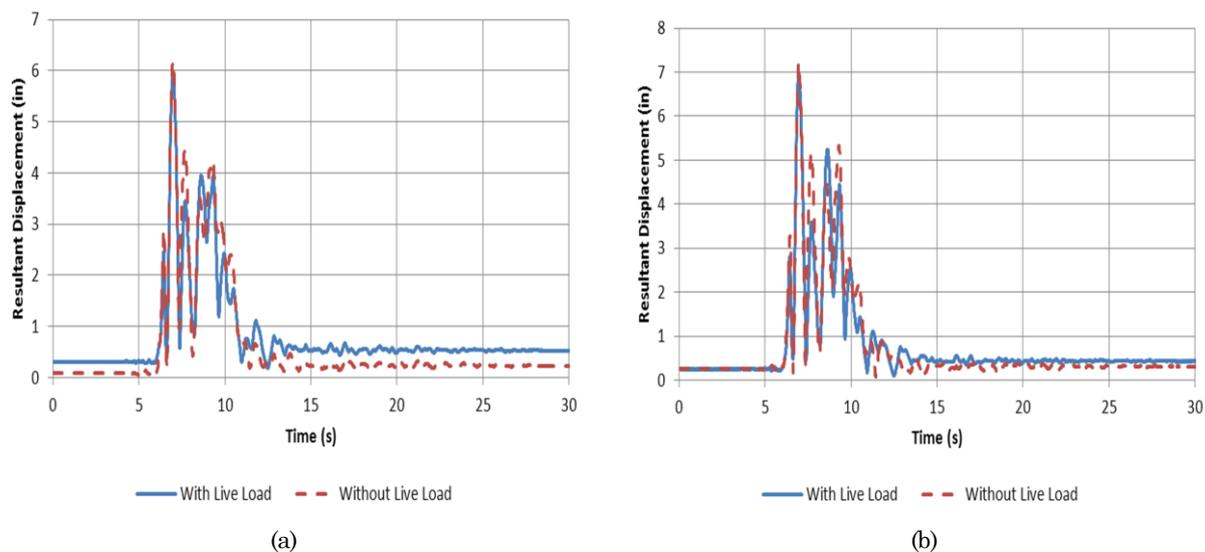
Figure 8. (a) North and (b) South Column Absolute Displacement Histories during 250% DE Run
