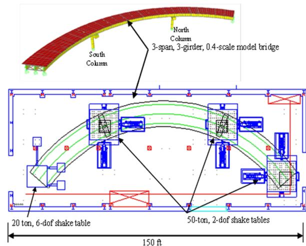
**Figure 1.** Bridge Model and Layout in Large-Scale Structures Laboratory
