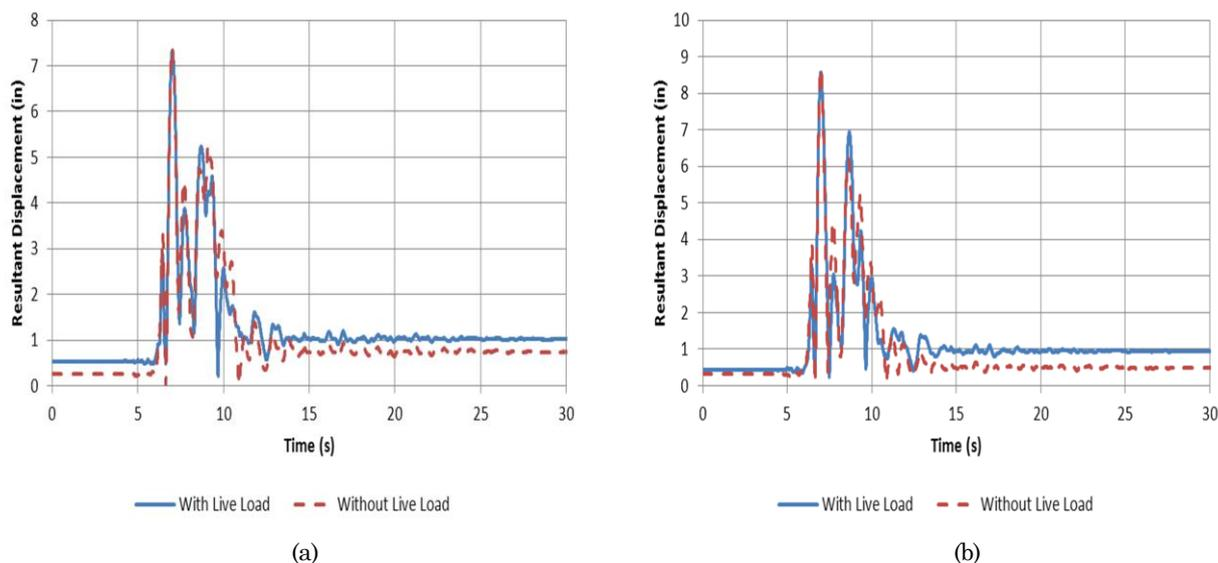
Figure 9. (a) North and (b) South Column Absolute Displacement Histories during 300% DE Run
