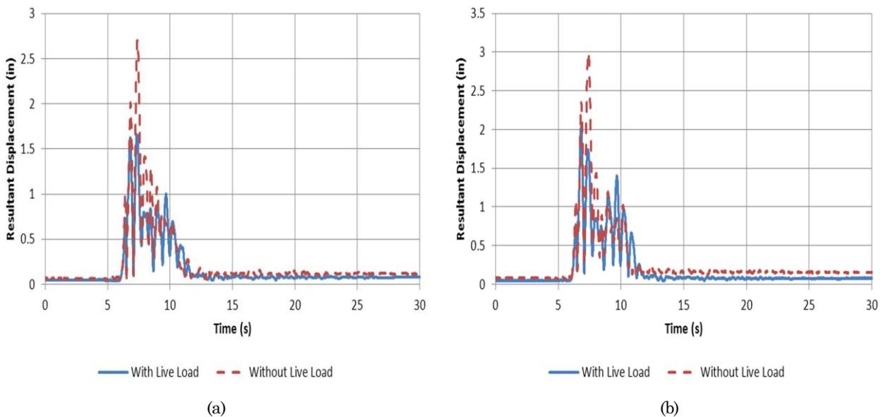
**Figure 7.** (a) North and (b) South Column Displacement Histories during 100% DE Run
