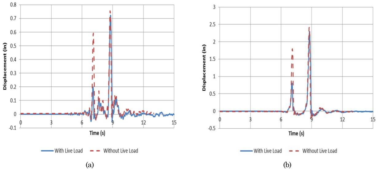
Figure 12. North Abutment's (a) Outer and (b) Inner Bays Displacement Histories during 350% DE Run
