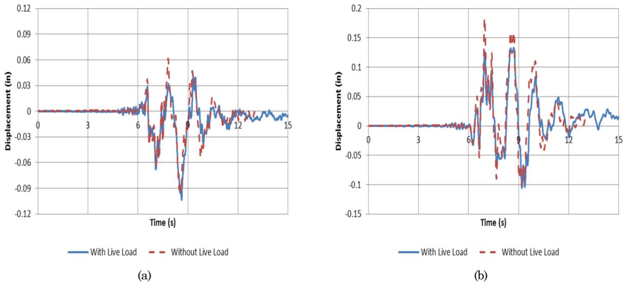
Figure 13. South Abutment's (a) Outer and (b) Inner Bays Displacement Histories during 350% DE Run
