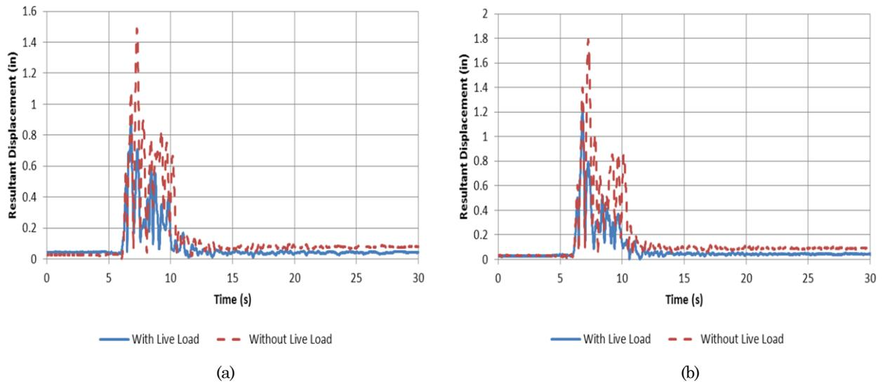
**Figure 6.** (a) North and (b) South Column Displacement Histories during 75% DE Run
